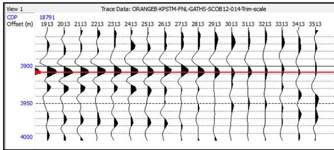
**Figure 3a** An example CMP offset gather from the SCOB-12 2D seismic survey near the Moosehead-1 well, SEG Negative polarity. Red line represents the Top Kudu Shale horizon location.
