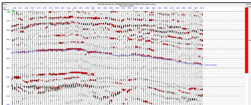
**Figure 3b.** Seismic stack showing AVA class4 anomalies highlighted in Red. Blue horizon is the Top Kudu Shale seismic pick.
