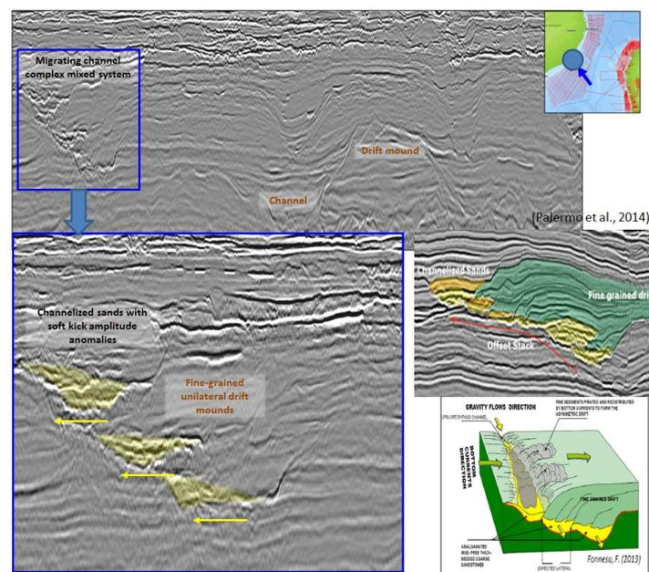
Figure 2: Strike line from the MOZ2D-17 survey showing different styles of hybrid systems.
