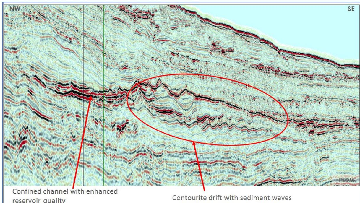
Figure 3: PSDM through a Barra well showing clear evidence for contourite drifts.
